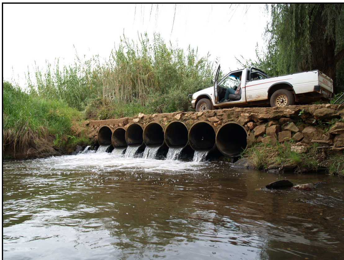
Photo 4 – The bridge where the flow in the Blaauwbankspruit leaving the Zwartkrans compartment was measured. Although the flow through the pipes was measured accurately, some water bypassed the pipes and flowed under the pipes. This volume was estimated by attempting to canalise it in parts into containers with known volumes.
